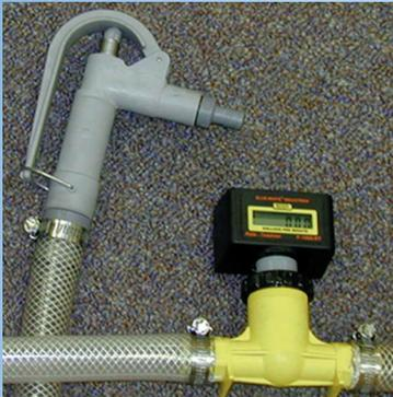
Use a Sethco polypropylene hand flow regulator to maintain accurate flow measurement when pump is turned off.
